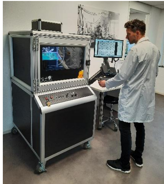
Figure 1. From its base in Helmond, The Netherlands, AQC B.V. provides highly complex PCBs to customers worldwide, relying on a Jewel Box T100 real-time X-ray inspection system provided by Glenbrook Technologies of Randolph, New Jersey, USA, to ensure quality.
