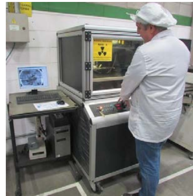
Sao Paulo-based EMS provider CADService has ensured assembly quality since 2008 with a Jewel Box 70T real-time X-ray inspection system supplied by Glenbrook Technologies of Randolph, New Jersey.
