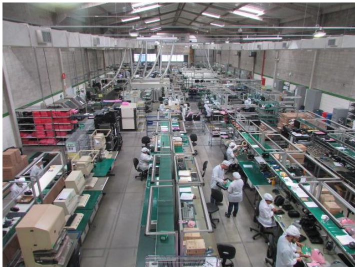
The factory floor of CADService in Sao Paulo, Brazil, where four automatic assembly lines can place up to 150,000 components per hour.
