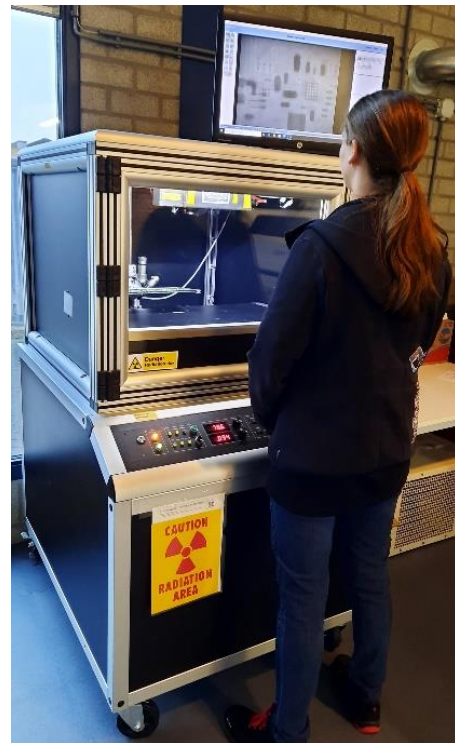
Figure 1: The Jewel Box 70T real-time x-ray system from Glenbrook Technologies helps support the development of new solder pastes at Cobar/Balver Zinn.
