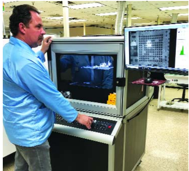
East/West's operators use Glenbrook's JewelBox X-ray system to inspect the integrity of solder pads underneath components.
